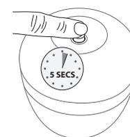
While the UV-C lamp shuts off automatically in 3-1/2 minutes, you may want to stop the cycle before it is complete. To do so, simply press and hold the LED power light for 5 seconds. The red light will go off indicating the cycle has stopped.
