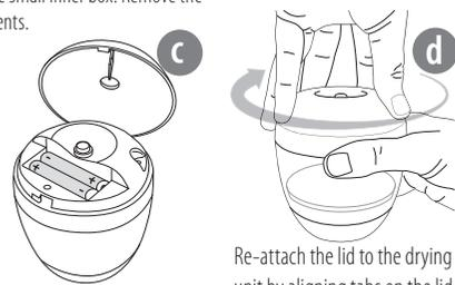
Install batteries with correct polarity.
