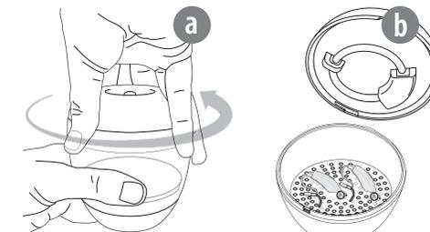
Remove lid and battery compartment sections by turning counterclockwise.
