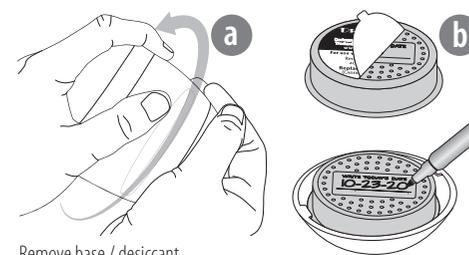
Remove base / desiccant compartment by turning counter-clockwise.
