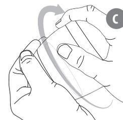
Re-attach the base to the drying unit by aligning tabs on the base with notches on the unit. Turn clockwise to close.
